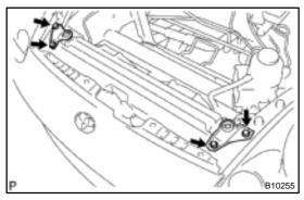
(b) Remove the 4 bolts and 2 radiator upper support.
