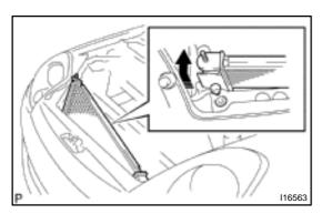
(c) Pull up the radiator right side, remove the bush at the bottom side of the radiator from the existing concave, and move it backword.
